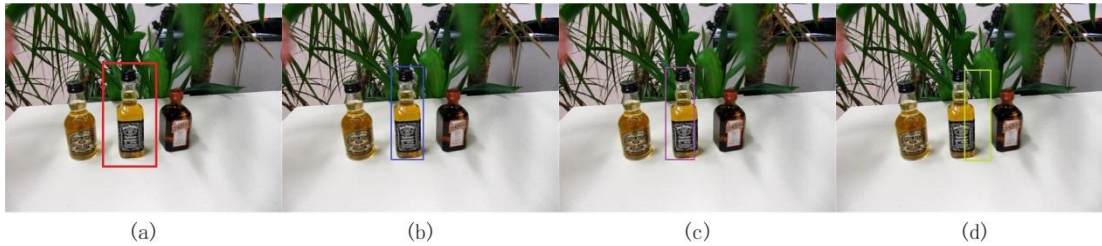
Fig2 (a) The red box is the candidate area. (b),(c),(d) are candidate area as the object probability. The probability that blue box(b) is the object is 0.73 .The probability that blue box(c) is the object is 0.51. The probability that blue box(d) is the object is 0.34.
